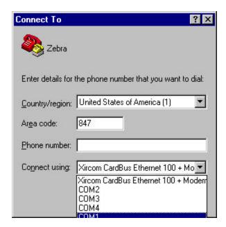
5. Hyper Terminal will then ask about the COM parameters. The Defaults for Zebra printers is 9600 baud, 8 data bits, 1 stop bit, no parity, and Xon\Xoff handshaking. Then click OK.
